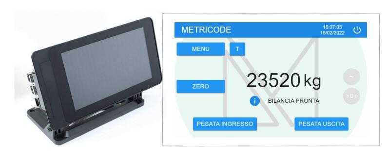
WeighIT EASY is the software which simplifies the management of the input/output weighs on the weigh bridge through the use of a touch screen display.
